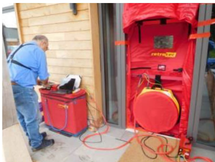
Figure 30: Air test being undertaken at Pippin Barn
