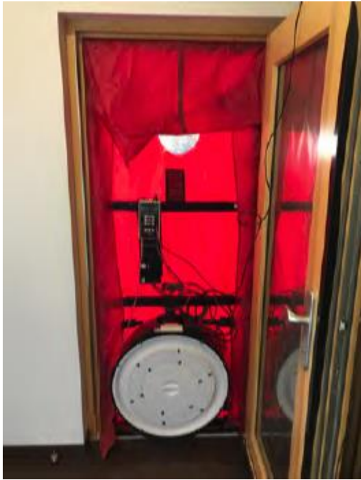
Photo of blower door test in progress
