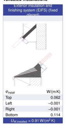
$<sup>^{1}</sup>$ Includes $\Delta U = 0.22 \text{ W/(m}^{2} \text{ K)}$ . Determined through 3D FEM simulation
