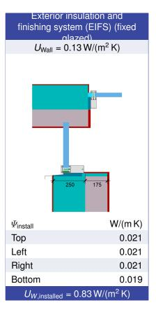
$<sup>^{1}</sup>$ Includes $\Delta U = 0.17 \text{ W/(m}^{2} \text{ K)}$ . Determined through 3D FEM simulation
