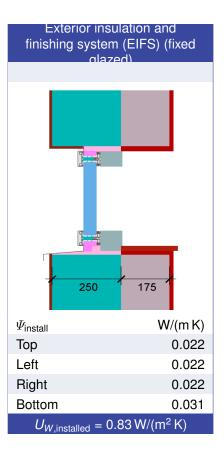
$<sup>^{1}</sup>$ Includes $\Delta U = 0.26 \text{ W/(m}^{2} \text{ K)}$ . Determined through 3D FEM simulation
