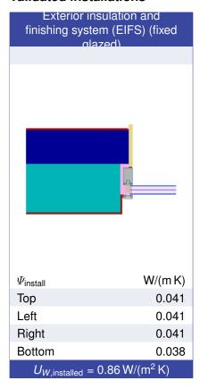
$<sup>^{1}</sup>$ Includes $\Delta U = 0.12 \text{ W/(m}^{2} \text{ K)}$ . Determined through 3D FEM simulation
