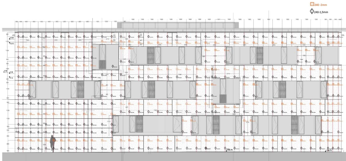
Installation-plan reference facade of the certified component
