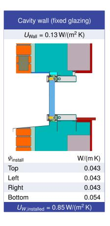
$<sup>^{1}</sup>$ Includes $\Delta U = 0.19 \text{ W/(m}^{2} \text{ K)}$ . Determined through 3D FEM simulation
